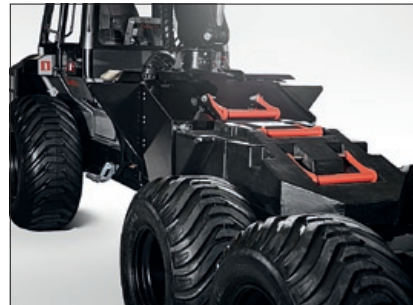
Two counterweights around 1100 kg each and a spacious storage box.
